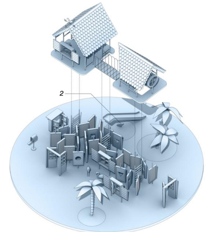
Fig. 5: Axonometric showing reconfigured panels and relationship to upper deck
